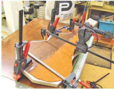
▲ Pic.8 Edge-joint the two pieces of the back. Only gentle clamping pressure is required with such thin stock
